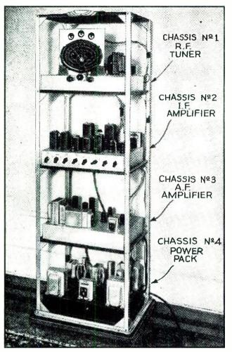
Fig. K. Front view of all chassis of completed 30-Tube Set.
