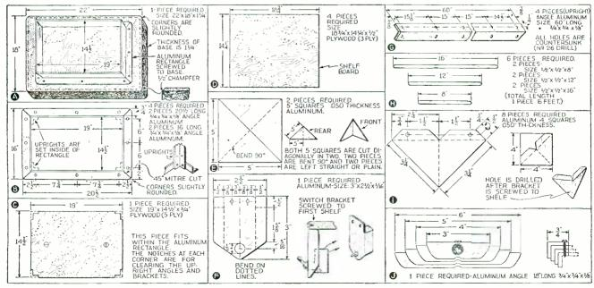
Fig. 18. Here are the steps necessary to construct the rack for the 4 chassis. These specifications must be followed exactly if the chassis are to fit.
